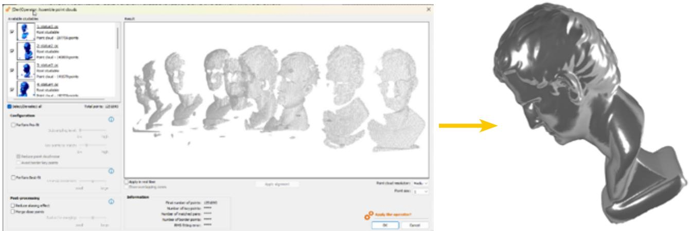
**Above.** Multiple point clouds can now be stitched into a single point cloud converted to Shells for metrological analysis
