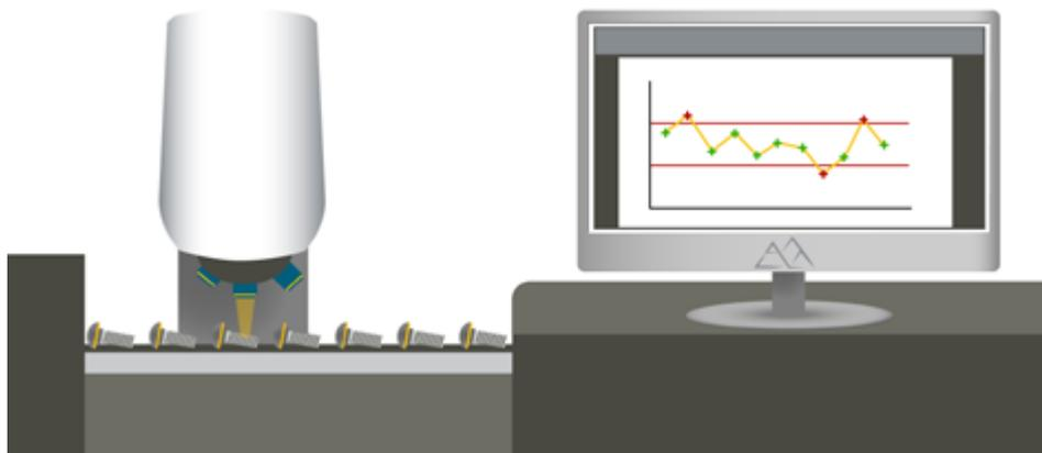
**Left.** In continuous production environments, every time a new measurement is performed, results and statistical studies are automatically updated.
