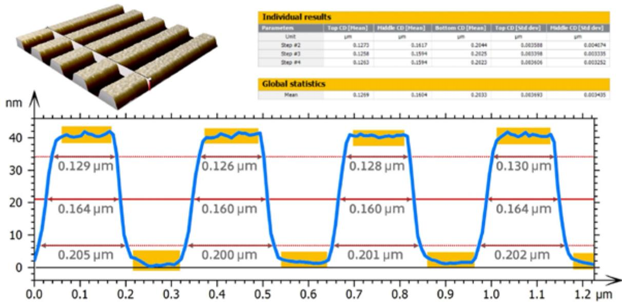
Above. New Critical Dimensions study for analysis of semiconductor fabrication processes.
