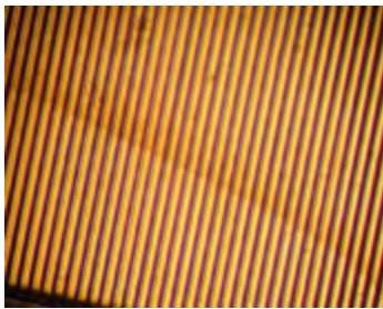
Stain on a sinusoidal profile with R_a = 3 \mu\text{m}
