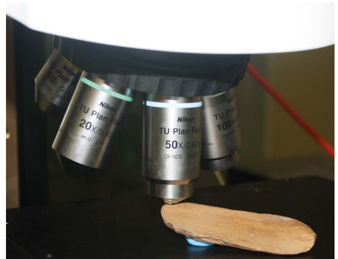
Hide working stone tool analyzed with the Sensofar S-Neox
