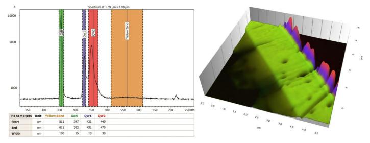
Visualization of spectroscopic features on a gallium nitride light emitting diode (LED) obtained by Attolight's high resolution cathodoluminescence technology. Left: band definition in AttoMap software; each band is associated to a relevant spectral feature (band edge, quantum wells, impurities). Right: 3D image of spectroscopic bands in AttoMap.
